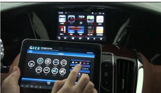
Figure 9. Using the Pad to turn up the volume, and the volume is 15.
